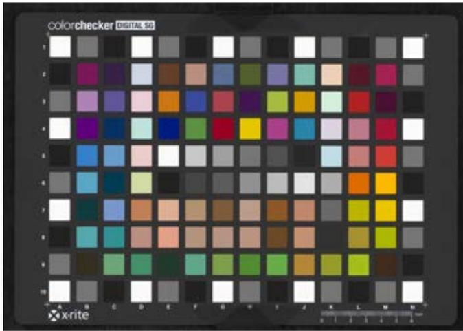
*This is the ColorChecker SG target we photograph to build the input profile. It consists of 140 color patches. This target has become the industry standard for building camera and scanner profiles.*
