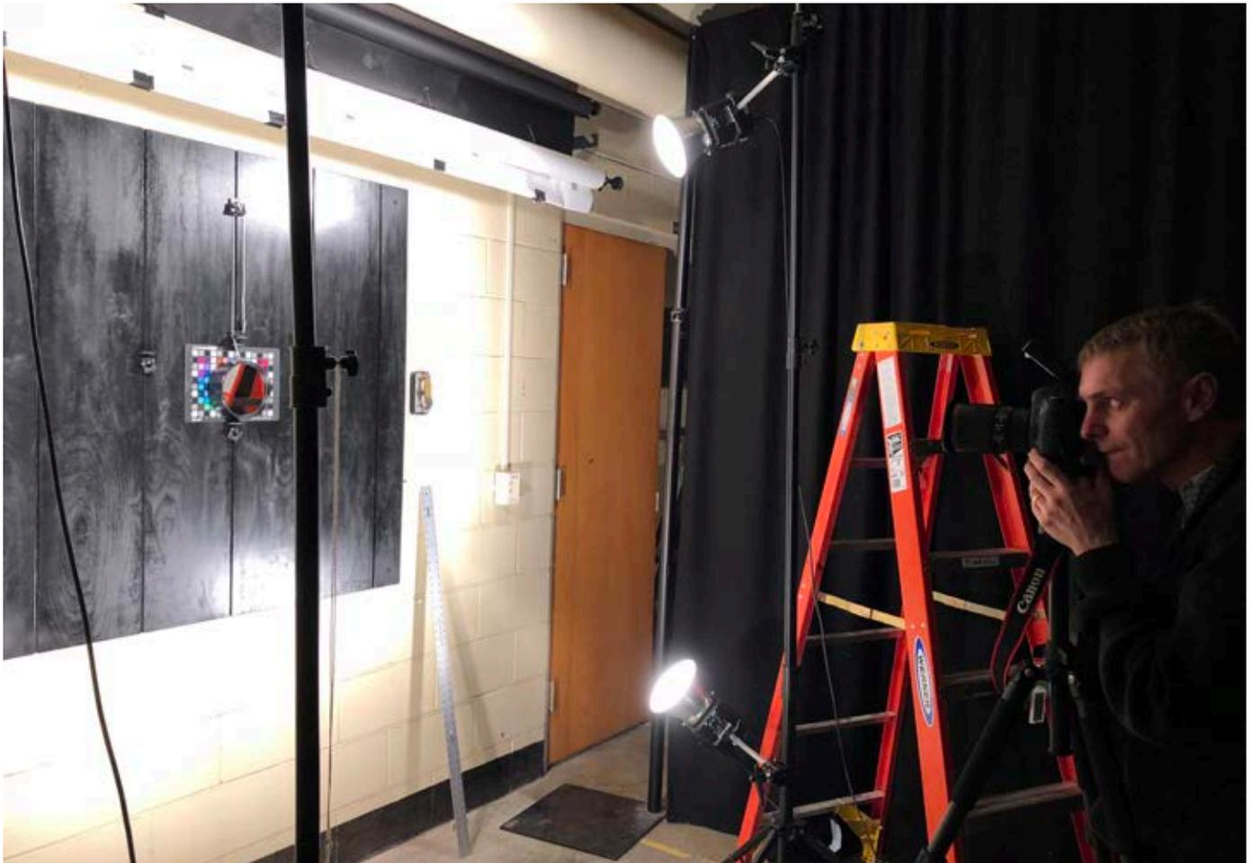
Here, Professor Van Kleeck positions the camera using the Hasselblad photographic mirror and the Zig-Align mirrored filter on the camera. You can also see the Einstein strobe lights mounted on the two parallel light stands. The ColorChecker SG is behind the photographic mirror.
